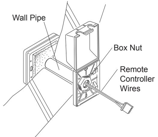
2. Drill a  $\varnothing$  1-1/4" hole in the wall where the remote controller will be installed.
