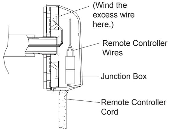
3. Insert the wall pipe containing the remote controller wires through the hole.
